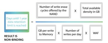
If based on this tentative calculation the lifetime of the e-MMC under a given usage scenario is not sufficient in relation to the expected life time of the product there are options to improve the situation A) Use the "Enhanced User Data Area" or so called pseudo-SLC. This will increase the available write erase cycles from ~3K to up to ~max.20K (@40 °C). Note: This will halve the available density.
