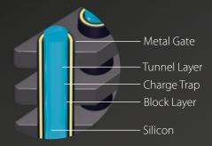
Our cutting-edge 3D BiCS FLASH technology with 64- and 96-layer stacking make a powerful memory solutions possible. It gives BiCS FLASH far higher die area density compared to 2D NAND. BiCS FLASH reduces the chip size by optimizing both circuit technology and the manufacturing process.
